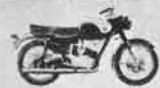
For The Sports Enthusiast YAMAHA's Famous 250-S Twin Cylinder 23-hp 5-speed road model
