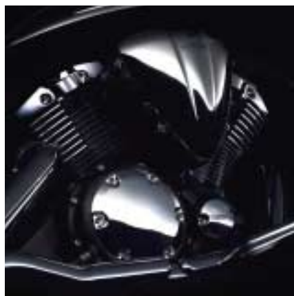
With the new-design liquid-cooled engine, the balancer helps accentuate the sense of pulse, and so does the noise absorbing function of the liquid cooling system
