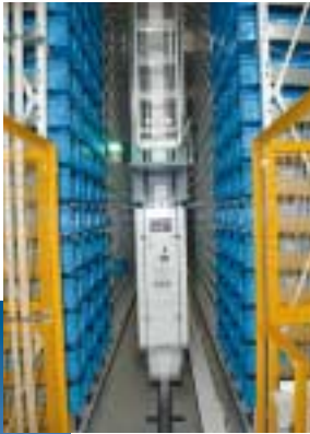
The AS/RS (Automated Storage & Retrieval System) has approximately 100,000 locations
