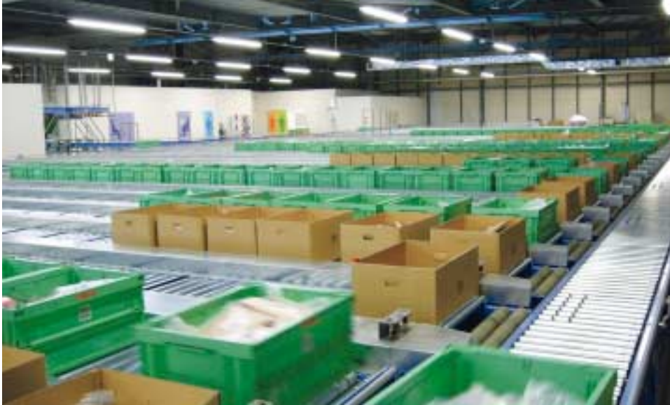
The order merge line facility located on the facility's 2nd floor consists of 40 lines
