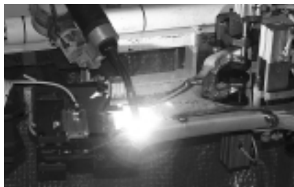
The YZ 125/250 frame is made up of 13 aluminum parts that are welded together in over ten different steps, with most of the welding done by carefully programmed robots
