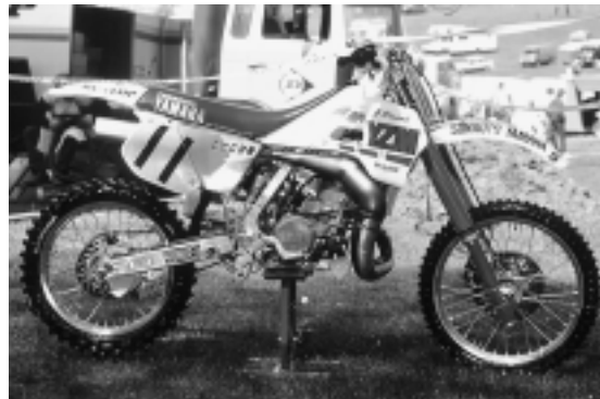
Yamaha began exploring the possibilities of aluminum frames on motocrossers 18 years ago. The YZM500 entered in the 88' VMX
