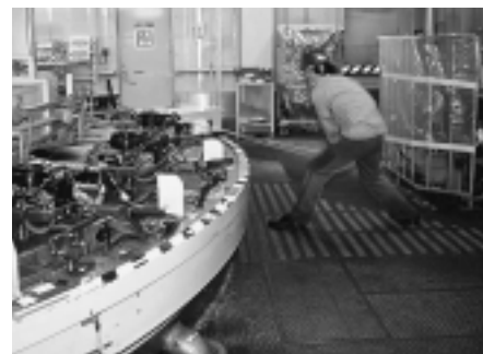
Yamaha Enduro outboards are tested in all types of simulated environments during the development process. They are tested with a variety of different types of fuel and prototypes are made to test in the actual markets. Also, data is taken and tests made for other factors like oil types, different air and water temperatures and the amount of calcium in different sea water environments. This photo shows final product testing
