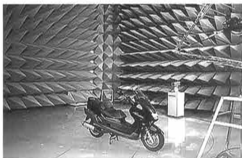
A scooter is tested in the "Yamaha Motor Electromagnetic Environment Experiment Room"
