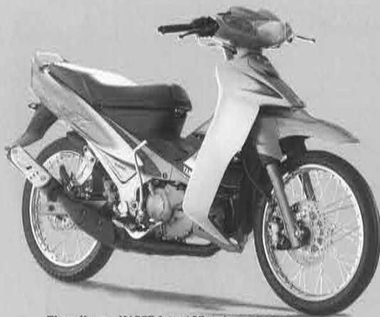
The all new Y125Z is a 125cc two-stroke under-bone model with a catalyser that meets the Euro-1 emissions standard
