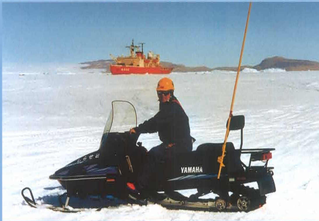
Yamaha VK540E2 snowmobiles like this are used for ice sample collection and personnel transport
