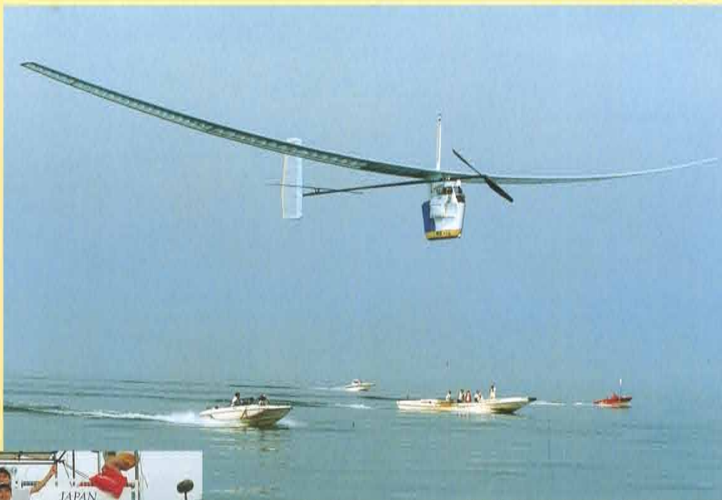
The Gokuraku Tombo (super happy dragonfly), its high-tech carbon fiber wings bent in flight, on the way to a Japanese distance record
