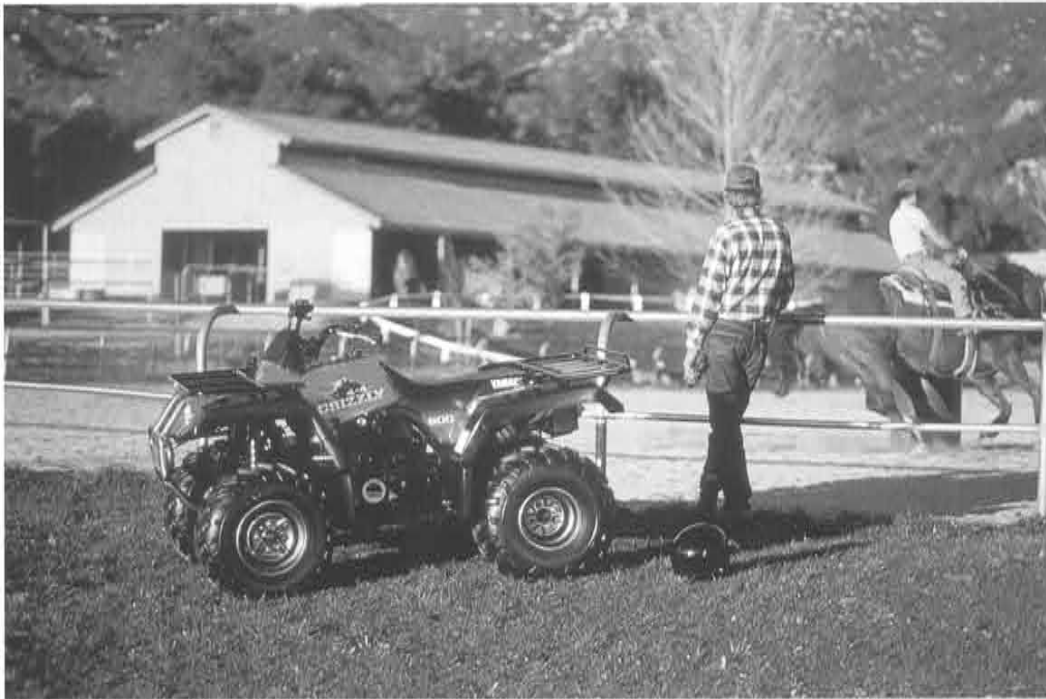
The Grizzly features a straight-line design based on military vehicles with special high-grooved, 25-inch Dunlop tires
