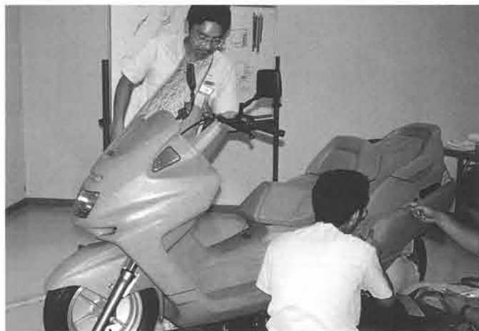
Entering the clay model mock-up stage, representatives of the Manufacturing Division joined in the development process. To ensure side-wind stability, tests were conducted in the wind tunnel, and windscreens angle and shape were checked repeatedly
