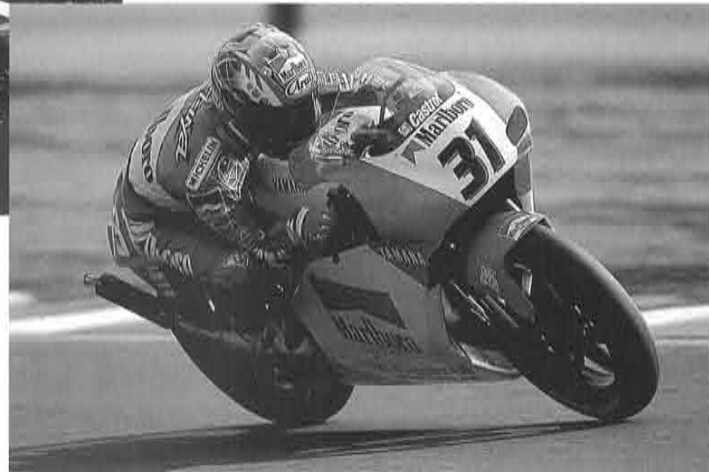
Tetsuya Harada on the newly developed '96 YZR250 with a redesigned rear cowl that improved aerodynamic characteristics
