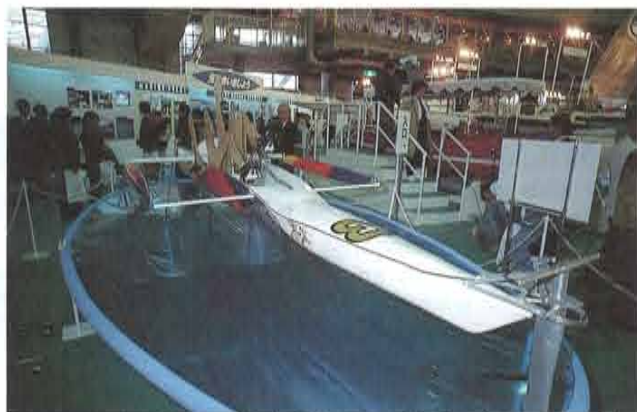
A man-powered pedal-operated hydrofoil boat, one of the Yamaha concept models.
