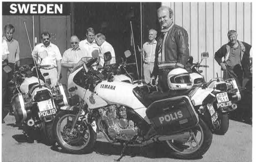
SWEDEN The first policeman picks up his new Yamaha XJ900 at the offices of Swedish importer Hallman & Enequist. The Swedish Police version of the XJ900 features a radio system, special lights, saddle bags and a unique "safety-look" color stripe.
