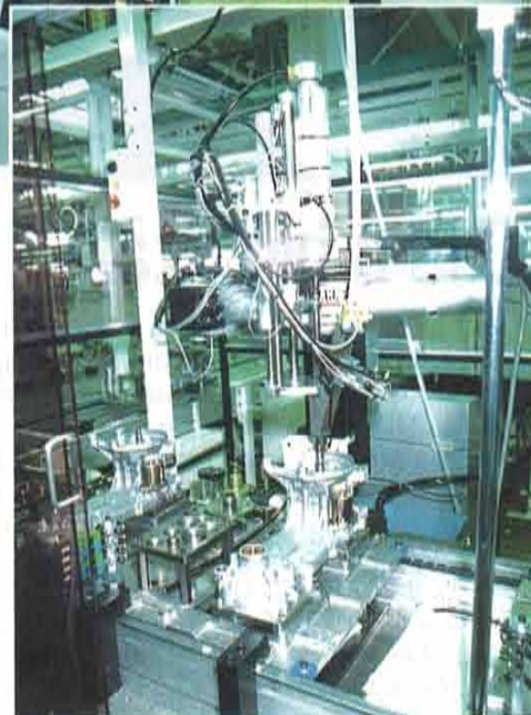
A close-up of one of the assembly robots. The robot is assembling a crankcase.
