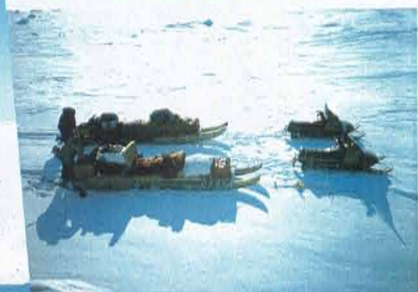
The Yamaha snowmobile Excel III proved extremely tough and reliable over the ice floe. The 2-stroke twin 340cc engine got enlivened in the severe cold sinking as low as 40°C below zero. Each machine covered a total of over 1200km without trouble. "It showed a wonderful performance while getting through an upheaved ice zone. Towing a 450kg sleigh it worked hard", says Masako.
