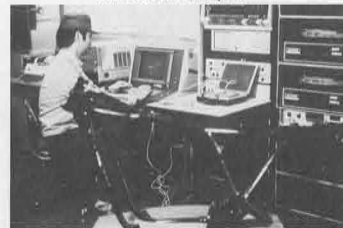
The strength and rigidity of individual component parts are computer-analyzed.
