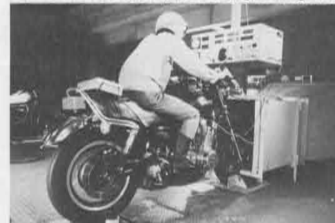
A turbocharged engine is tested for its max. power output, torque development and general power characteristics to realize an ideal engine setting.
