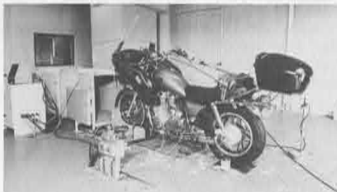
Machine's durability is thoroughly tested here. Every conceivable riding condition is artificially prepared.
