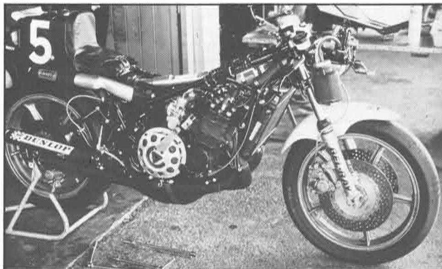
The Sonauto Yamaha T2750 is fitted with a kick starter.
