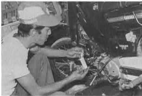
Spark plug inspection
