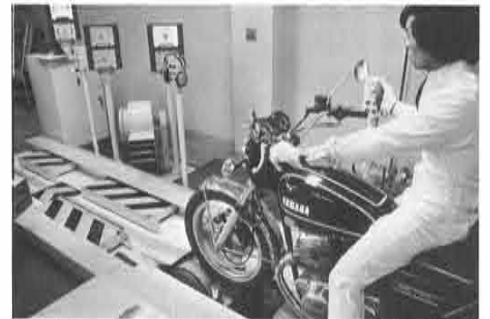
Braking power and rear wheel output are tested here
