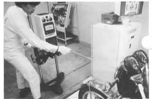
Wheels are tested for correct alignment
