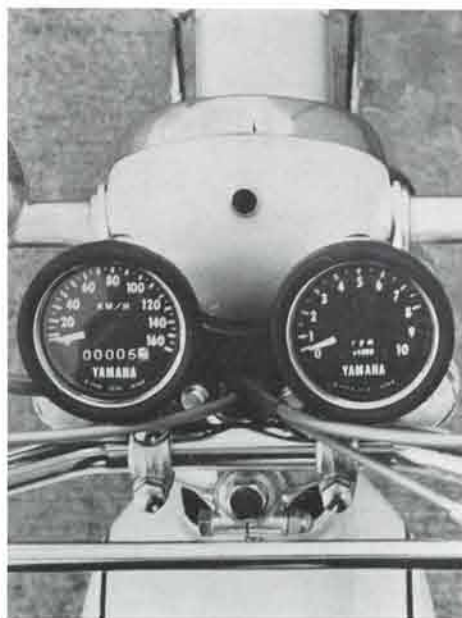
Independent tachometer and speedometer. Large-sized flasher lamp makes for safety in urban riding.
