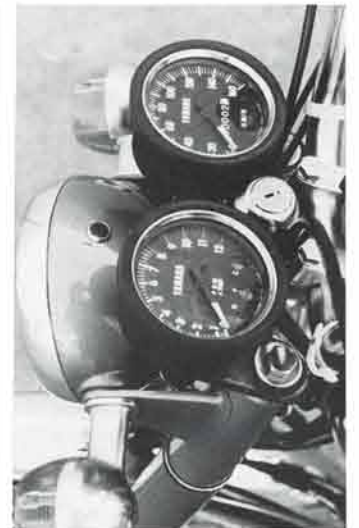
Main switch is placed in an easy-to-operate position. Light switches are gathered on left handle.
