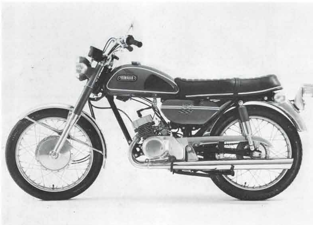
Main switch is placed in an easy-to-operate position. Light switches are gathered on left handle.
