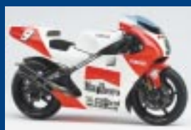
OWJ1 (1996) Adoption of a powder-metal piston This model featured the powder-metal piston with enhanced heat resistance as well as a new frame design that eliminated the seat rail. Norick Abe rode this machine in the Japan GP and scored his first GP win.
