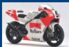
OWF9 (1994 ~ 1995) Forced-air type air box boosts intake performance On this machine, L. Cadalora ranked second overall for the season. In the 1995 model, an air type air box was introduced to boost intake performance.
