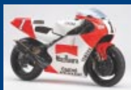
OWF2 (1993) Introduction of an extruded aluminum frame The aluminum main frame of this model was made of extruded aluminum with a segmented box cross-section. This design helped Yamaha win its eighth manufacturers title.
