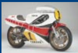
OW54 (1981) Featuring the square-4 rotary valve engine format
