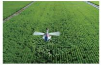
Aerial agrichemical spraying using unmanned helicopter
