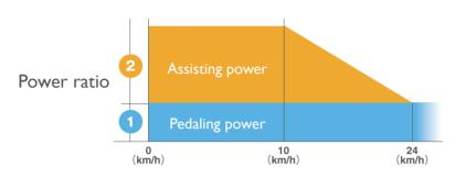
Up to 10 km/h, electric power assists pedaling at a maximum ratio of 1:2\* Above 10 km/h, electric power assist
