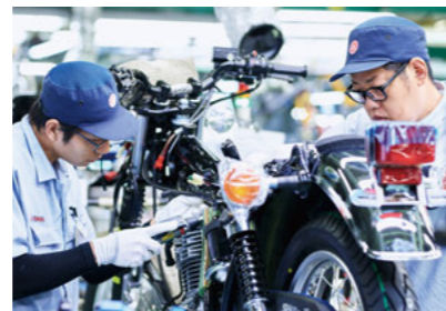
Our long-selling SR400 model is assembled through "cell manufacturing" in which the entire motorcycle is put together by a two-person team.
