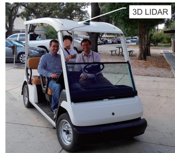
Figure 3. Low-speed automated vehicle equipped with the VGL system
