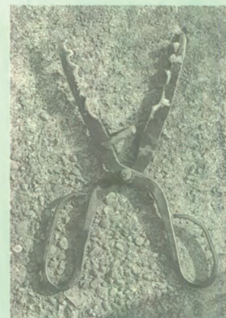
Scissors for holding the eel. The blades are notched to prevent slipping.
