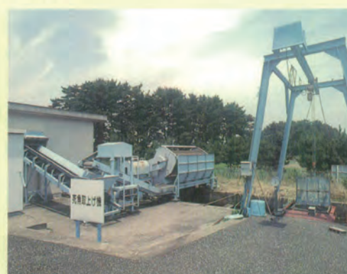
A dead fish removal device
