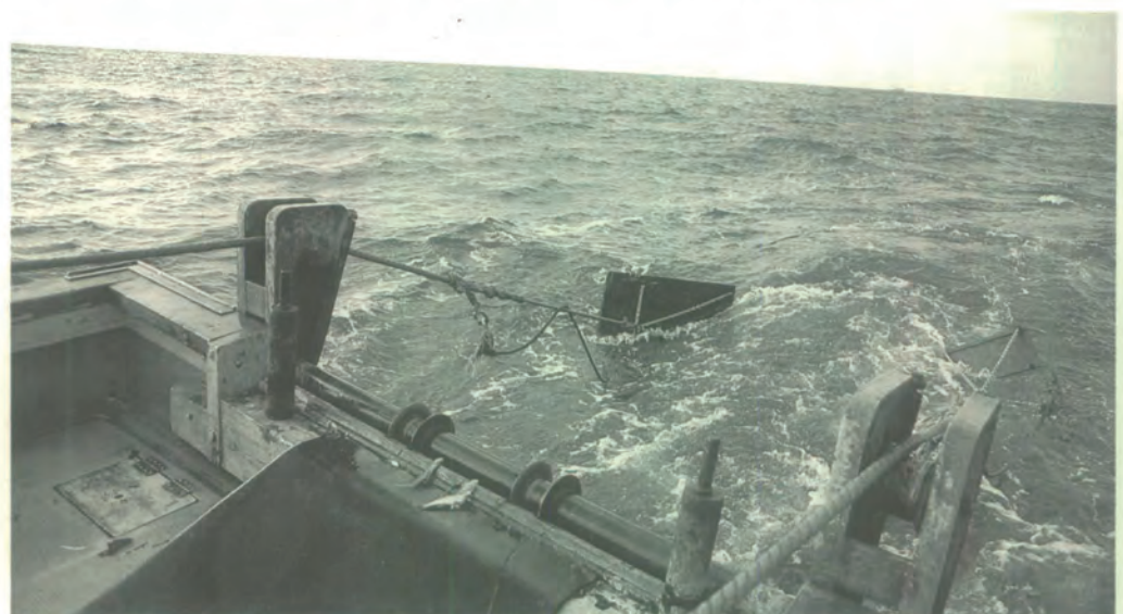
In some parts of east Japan, circular otter boards are popular (photo courtesy: Institute of Fisheries Engineering Research)
