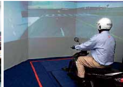
Motorcycle simulator that allows students to experience various situations without risk
