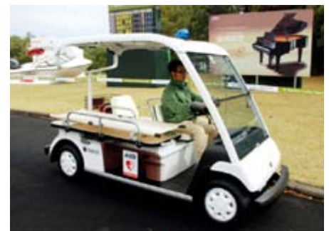
The golf car based ambulance is outfitted with an AED, stretcher and other specialized equipment.
