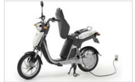
The EC-03 is an electric motorcycle released in Japan in autumn 2010; it adopts a plug-in charging format, allowing the battery to be recharged at home or away
