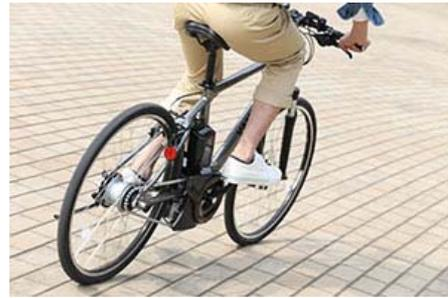
The electrically power assisted bicycle is a vehicle that didn't exist anywhere in the world until Yamaha Motor developed and marketed it in 1993. By mounting a small electric motor and battery to provide a power assist to the force applied to the pedals by the rider, thus addressing the weak points of a bicycle such as the heavy load of pedaling uphill or into the wind, made riding much easier and more enjoyable.
