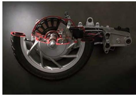
The super-thin power unit of the Passol integrates the brushless DC motor, controller, transmission and a drum brake all into the rear wheel hub.
