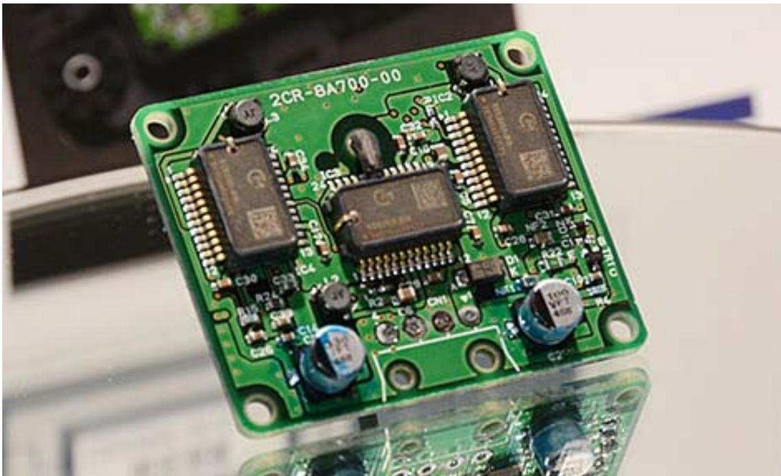
The 6-axis Inertial Measurement Unit (IMU) used on the new YZF-R1
