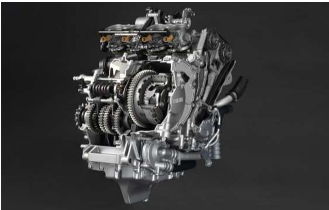
A cutaway of the new YZF-R1's 998cc liquid-cooled in-line 4-cylinder engine with a crossplane crankshaft
