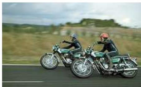
Drawing on its expertise garnered in the joint development of the Toyota 2000GT sports car, Yamaha developed and marketed in 1970 its first 4-stroke model in the XS-1, a large-displacement sport model with a lightweight, slim and compact design.
