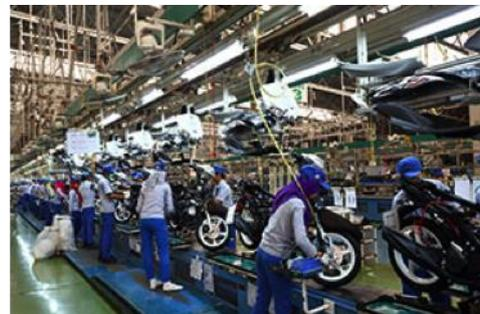
This “divided workflow assembly line” in Indonesia increases efficiency by eliminating any need to turn around while working. This waste-free production method was first perfected at the Iwata Main Factory and is now used in many overseas group factories.
