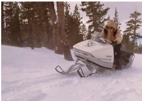
Yamaha's first snowmobile model, the "SL350." Statistically, it had a maximum output of 20 hp, a top speed of 60 km/h, could climb an incline of up to 25 degrees and pull a 500 kg load (1968).
