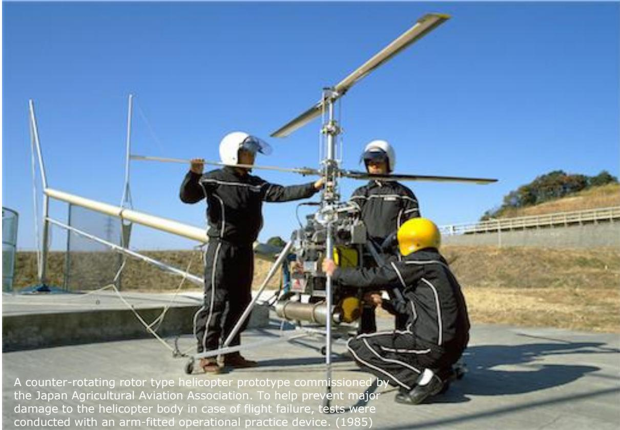
A counter-rotating rotor type helicopter prototype commissioned by the Japan Agricultural Aviation Association. To help prevent major damage to the helicopter body in case of flight failure, tests were conducted with an arm-fitted operational practice device. (1985)
