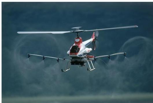
Crop spraying with the "R-50" industrial-use unmanned helicopter. This photo shows how downwash from the main rotor helps distribute the spray of agrichemicals. The sprayers and other components mounted are all specially developed for each body type to further increase operational efficiency.
