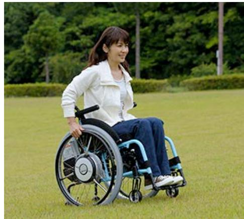
As successor to the JW-II unit released in 1996, the new “JWX-2” makes full use of Yamaha PAS technology to enable assist setting adjustments to fit individual user strength and/or preferences and achieve smoother, more natural performance, etc.
