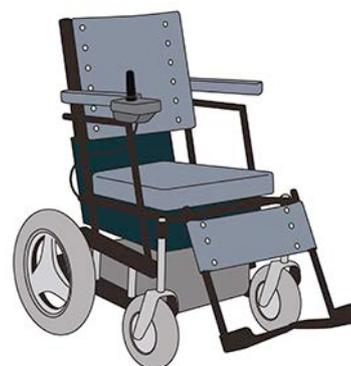
Conventional electrically powered wheelchairs from other companies had the drawbacks of large, integrated motor and battery assemblies that limited design freedom even in custom-made models, and were heavy at about 80 kg
