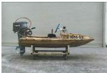
A new prototype embodying the project's new keywords of "sit-down type" and "tandem model" was immediately developed. Initial R&D was carried out with the prototype mounting an outboard motor.
