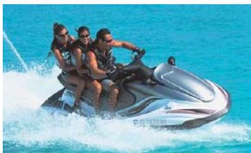
The world's first 4-stroke engine PWC, the "FX140" (2002) cleared the U.S. Environmental Protection Agency's emissions standards.
