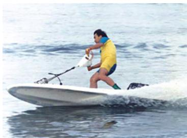
The "Power Ski" prototype model tested in the U.S. in 1984 was a stand-up type powered by the engine from a 25 hp outboard motor.
