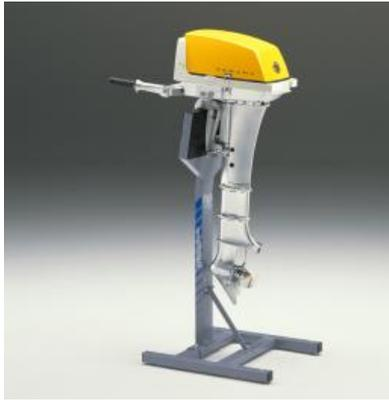
The first Yamaha outboard motor was the "P-7" (1960). It mounted an air-cooled, 2-stroke 123cc engine and was designed to power the wooden boats of the day.
