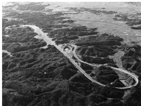
The Fukuroi Test Course where many historic Yamaha motorcycles have been developed over the years was completed in 1969. Built on 370,000 m<sup>2</sup> of land, the 5.24 km long course has an underpass, a 1.4 km long straight, a 7.9% incline and more. This layout was chosen to allow for testing a wide variety of conditions.
