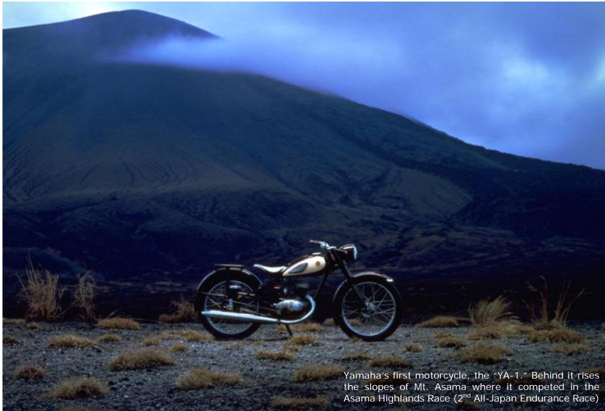
The first Yamaha motorcycle was the "YA-1" (1955) powered by a 2-stroke, single-cylinder 125cc engine.
