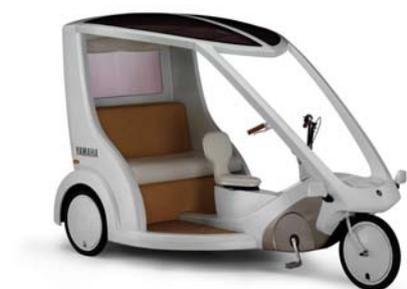
This Yamaha-built bicycle taxi gained much attention in its use as a transporter at the 2005 World Exposition, Aichi, Japan. It used a PAS drive unit and the body was made of the same fiber reinforced plastic Yamaha successfully employs in manufacturing its boats and golf cars.
