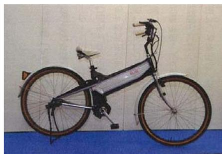
An early prototype electrically power assisted bicycle.
