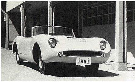
For the YX-30 (Type I) prototype completed in 1960, Yamaha succeeded in developing the world's first all-aluminum engine. In track tests, the car recorded a top speed of 144 km/h.
