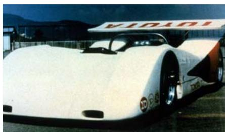
The "Toyota 7" was developed to the specification of the "Group 7" class of international endurance racing for 2-seater cars powered by large-displacement engines. It went on to be a top contender in various race classes in Japan.
