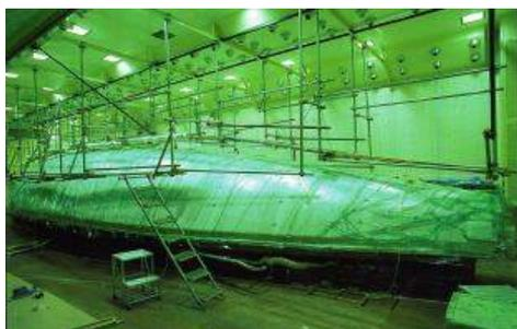
Yamaha put its hull-building skills to the test in constructing its first ever carbon composite body for the *Nippon Challenge* race boats
