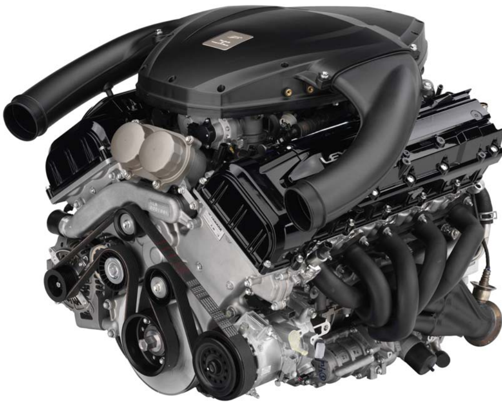
The 1LR-GUE engine mounted on the LEXUS LFA
