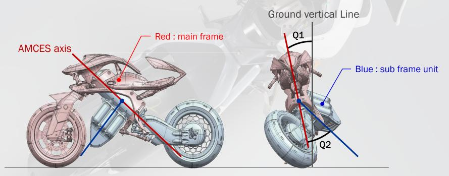
The basis for MOTOROiD's balance control is the inverted pendulum, where using the information of the angle between the axis perpendicular to the ground and the vehicle inclination, Q 1, and the inclination of the pendulum, Q 2, the actuator controls the vehicle's self-balancing function.
