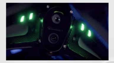
A facial recognition system gives MOTOROID the ability to respond only to its owner. It is also able to recognize gestures, making it possible for MOTOROID to also respond to hand movements, such as using a beckoning wave or a raised palm to instruct it to start or stop moving. The system's data is continuously sent to the control unit, where it is collected and used as feedback for controlling the machine.
