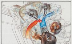
The FZ600's air-cooled, 598cc, DOHC engine has high-lift camshafts that act directly on the valves for maximum efficiency. It's also the narrowest engine in its class. Which means it accommodates lean angles unthinkable on ordinary motorcycles.
