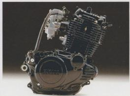
A single 350cc cylinder pumps out loads of hill-climbing torque.
