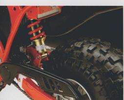
Race-proven Monocross rear suspension utilizes a single shock.
