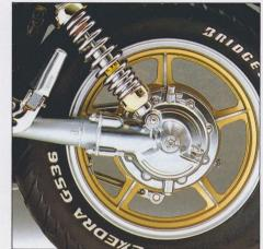
Transmitting the untiring power of the Virago 1100 engine to the rear wheel is no small task. A remarkably efficient shaft drive does it in style: totally enclosed, it is quieter than a chain and virtually never needs maintenance or replacement.
