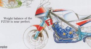
Lightweight half-fairing is wind tunnel-sculptured to combine aerodynamic efficiency with maximum rider comfort at speed. It is mounted directly onto the frame to eliminate weight inertia effect on the steering.
