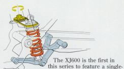
shock chassis. Yamaha's famous rising-rate Monocross system uses a box-section, high-tensile steel swinging arm. Its movement is controlled by lightweight linkage arms and a De Carbon-type gas/oil shock absorber with remote spring pre-load adjuster. This system gives progressive resistance to road shocks, low centre of gravity and centralized weight mass.
