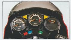
Full, easy-to-read instrument panel is mounted on to the head fairing and includes large speedometer, electric tachometer, indicator lights and main ignition switch with steering lock.
