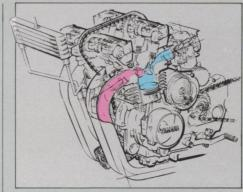
Compact, 4-cylinder, 598cc, DOHC engine features extra-large valves, extralight weight. Power-to-weight ratio is a "best in class" \*5.8lbs. per horse. Narrow design also gives you deep lean angles for hard cornering.
