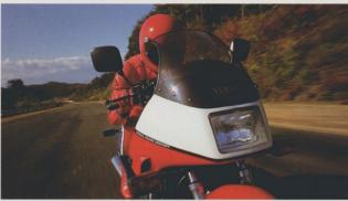
The correct aerodynamic profile is vital to a machine with the speed capabilities of the FJ1100. Therefore the bodywork of the Yamaha superbike has been developed as an integrated package: head fairing, engine undercowl with spoiler, wrap-around front fender and streamlined tail unit. All tested and proven in the wind tunnel.
