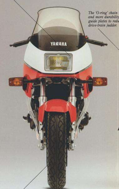
Triple-spoke, 16-inch wheels are used front and rear to reduce frontal area and lower the centre of gravity. Wide-profile, V-rated tyres put plenty of rubber on the road for traction and stable handling.
