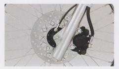
The disc brake has come to trail riding! The DT200 features a lightweight drilled disc, alloy calipers, semi-metallic friction pads and a plastic mudshield. The result is a brake that works perfectly in all conditions. Street or trail, wet or dry.
